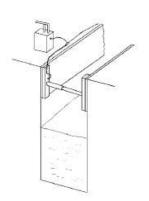
Release pressure on rams from top unit using the release tool and lift top unit from grave.
