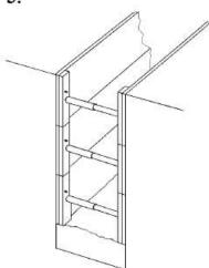
Release pressure from rams of uppermost unit by turning the valve on the pump, lift unit so that its top edge is level with the surface and repressurise rams to holding pressure.
