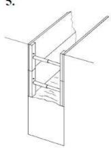
Release pressure from rams of uppermost unit by turning valve on pump, lift unit until its top edge is level with the surface of the grave and re-pressurise rams to holding pressure.
