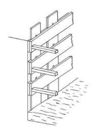
The piling timbers can be lifted one at a time so that their bottom edges are level with the top of the previously consolidated soil. The wedges are removed from **one** piling timber before it is lifted and are replaced immediately after repositioning. 4.
