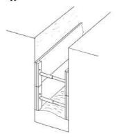
Attach lifting ropes to next unit and connect hoses to rams (if not already connected to dedicated hoses).
