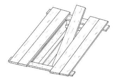
When backfilling large flints, pieces of rock or lumps of clay may damage the coffin when they impact from height. To reduce the risk of coffin damage a timber can be placed into the grave as shown in the above diagram. Backfill material will strike the timber, break its speed of fall and deflect to the sides of the grave.
