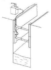
Connect two-way hose to rams of bottom unit placing hoses behind rams of top unit.
