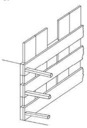
When close piling is incorporated **one piling timber** can be removed to aid ease of backfilling. This timber should only be removed to carry out the final stages of backfilling.
