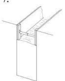
Release pressure by turning valve on pump and lift unit until its top edge is level with the surface of the grave. Re- pressurise rams to holding pressure. Remove hoses from rams.
