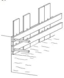
During backfilling operations the poling timbers will protrude from the grave to a height where difficulty may be encountered attempting to shovel soil over the tops of the piling timbers.
