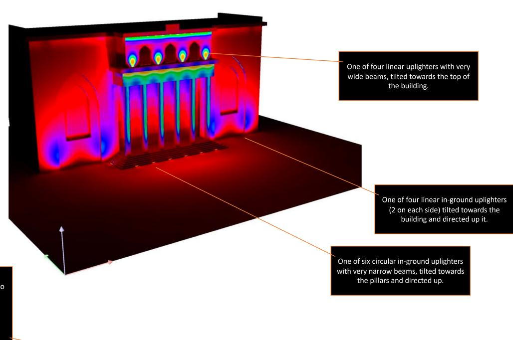
We drew a scale model of the Guildhall and simulated different lighting fixtures to check the effects.
