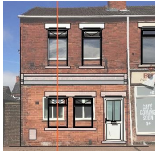
Preferred arrangement. Lower-floor windows aligned with upper floor and window heads are replicated.
