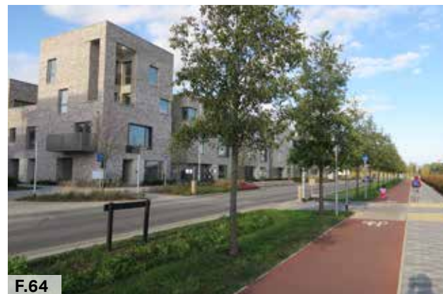
Figure 64: Example of a primary street with street trees and inset parking, Northwest Cambridge.
