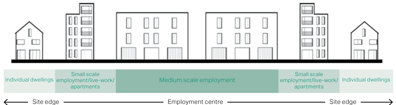
F.38 Figure 38: Section showing the transition from the employment centre to the residential site edge.
