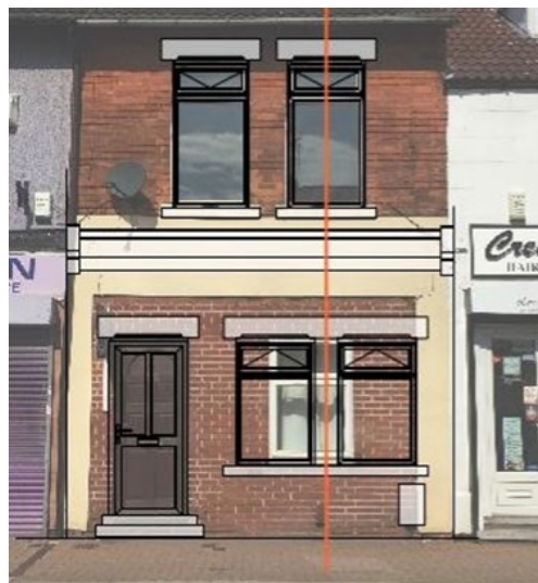
Preferred arrangement. Lower-floor windows aligned with upper floor and window heads are replicated.
